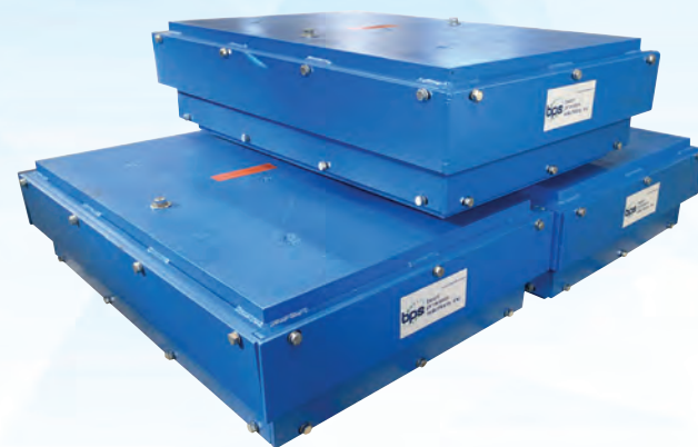
BPS shredder isolation mounts are designed to reduce vibration and shock from impact loading. These heavy-duty units are located between the main shredder assembly and the concrete support foundation.
